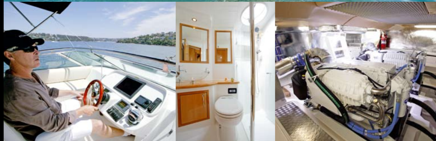
Top: The 55s have a lift-up transom RIB garage. Above, left to right: At the wheel of the A55s bridge helm; Heads have an overhead hatch for natural light and ventilation; Engine room is fully lined. Below: Saloon helm and galley.
